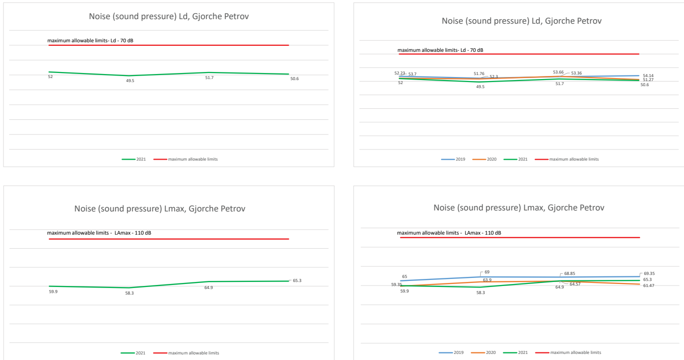
Graph 22: Noise measurement (Ld and LAmx noise pressure) at the Gjorce Petrov site in 2021 and comparison 2019 – 2021
