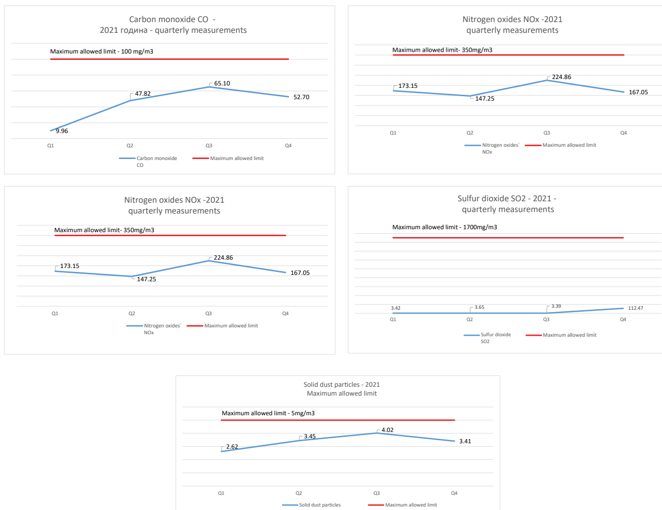
Graph 7: Quarterly measurements of air emissions (CO, NOx, SO2, and solid particles/dust) from the boiler room in Avtokomanda in 2021
